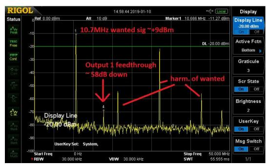
So, with buffering in these test examples, we get output level more suited to a double balanced diode mixer and improved suppression of the other channel by at least 10dB.
