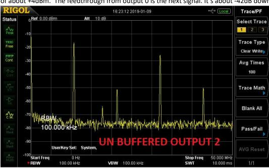
Next we check output 2 on the unbuffered board, below. The wanted signal at ~10.7MHz is at a level of about +4dBm. The feedthrough from output 0 is the next signal. It's about -42dB down
