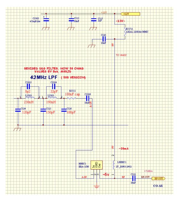
Fit the parts as per the Schematic, for the DDS output filter. NB: these must be the values for the 50R version of filter, as suggested by Bob, MORJD. See above.
