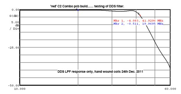
After fitting the ERA-1 amp, here is a sweep of the DDS filter plus the ERA-1 amplifier stage. (Note; there was a 30dB attenuator on the input, to prevent overload of the N2PK VNA used for the sweep)
