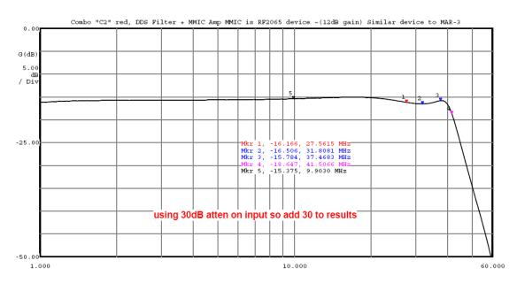
So, what is the end result of all of this? You should have no problems getting in excess of +7dBm output on all of the Bands up to 10M. It will drop slightly at 10M due to the fall of the DDS filter. (See plots above)
