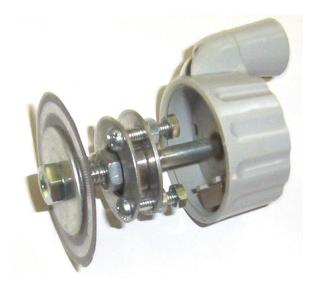
The shaft encoder is made with a roller ball bearing clamped between two Car mud-flap washers. The centers of two washers are drilled to 15mm diameter to allow space for the nuts that clamp the shaft (a bolt) onto the inner part of the roller ball bearing. Three 4mm diameter holes are drilled (120 deg apart) in each washer for three 4mm screws that are used to clamp the bearing between the washers and for mounting the shaft encoder to the front panel.
